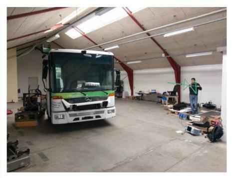
The truck was too large for SDU's EMC chamber why the pre-compliance test was carried out in a garage.
